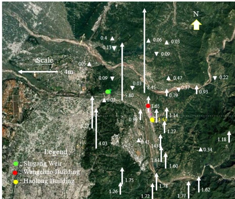
Figure 9. Vertical GPS velocity vector map during the 921 Jiji earthquake (After National Land Surveying and Mapping Center, 2002; Google Earth, 2024).
